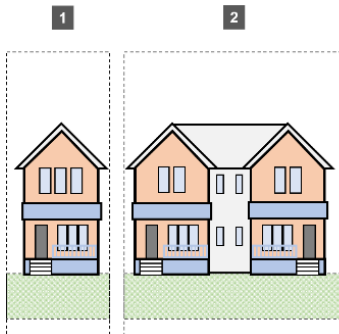
Figure 11 – Front Building Volume & Front Projection (Elevation View)
