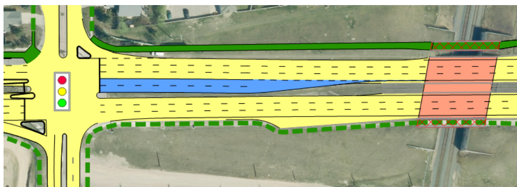
Figure ES 5.1: Dual WBL at Harvest Hills Way and CP Bridge
