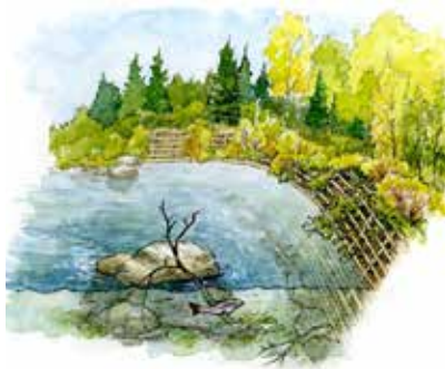
Bioengineering incorporates living and non-living plant materials in combination with natural and synthetic support materials.
